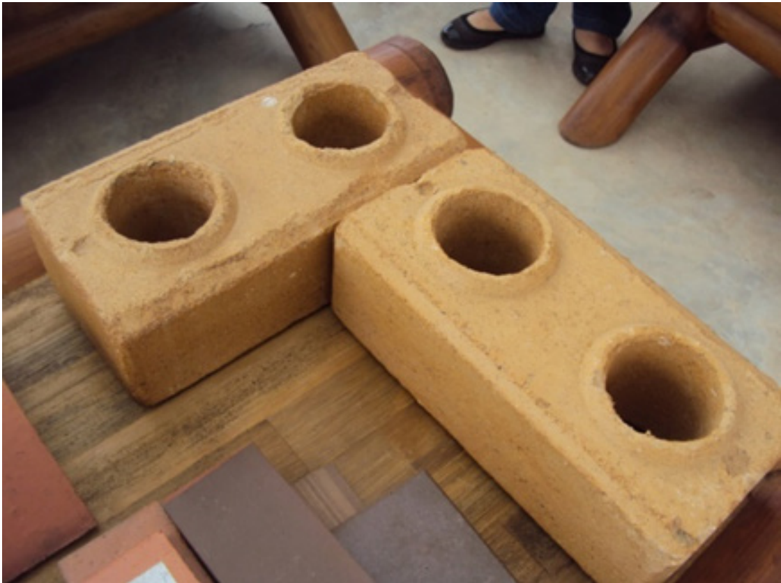
Figure 3. Soil-cement blocks manufactured using the CINVA-RAM
