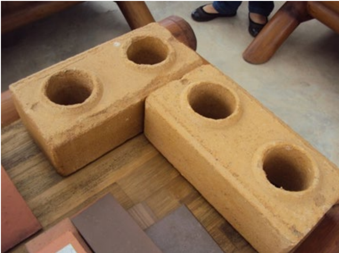
Figure 3. Soil-cement blocks manufactured using the CINVA-RAM
