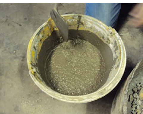
Figure 9. Pouring of fine aggregate into the mechanical suspension. Source: own elaboration (2019). CC BY
