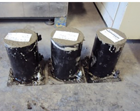
Figure 6. 10 × 20 cm cylindrical specimens (MCV). Source: own elaboration (2019). CC BY
