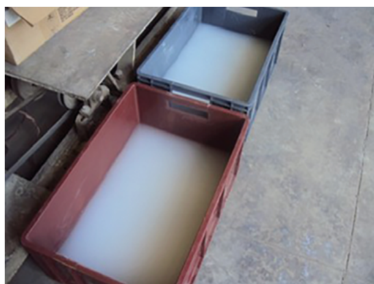
Figure 12. Preparation of lime water for curing. Source: own elaboration (2019). CC BY
