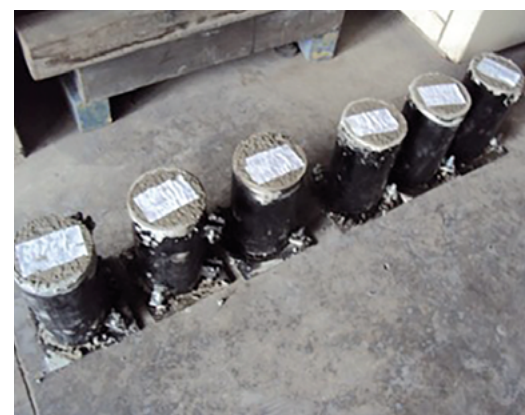
Figure 14. MCV and MSM specimens for seven-day failure. Source: own elaboration (2019). CC BY
