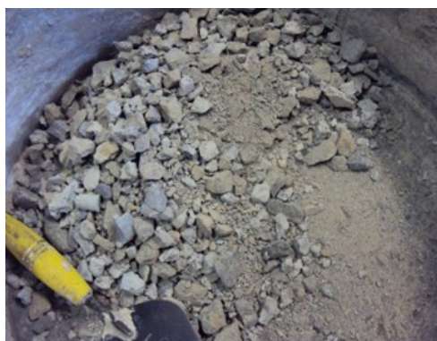
Figure 2. A mixture of coarse and fine aggregates in the dry state.
