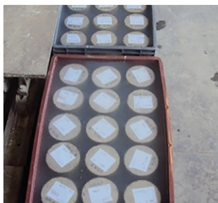
Figure 13. Immersion of the specimens for curing. Source: own elaboration (2019). CC BY
