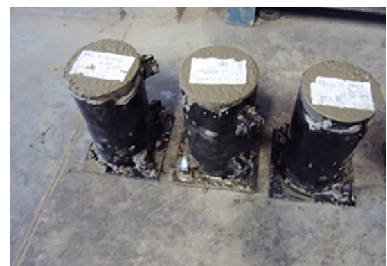
Figure 11. 10 × 20 cm cylindrical specimens (MSM). Source: own elaboration (2019). CC BY
