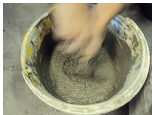
Figure 10. The coarse aggregate is mixed with the paste obtained by mechanical suspension. Source: own elaboration (2019). CC BY
