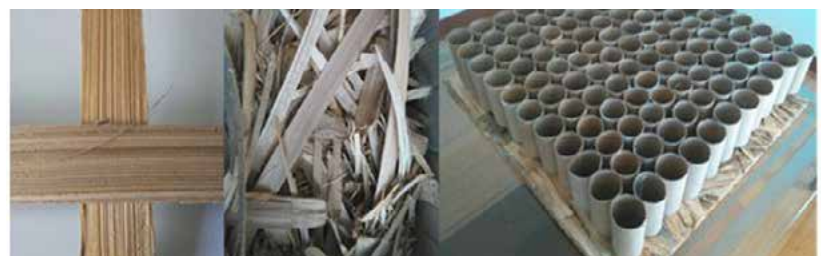
Figure 6. Recycled guadua fiber and recycled cardboard tubes Source: Own elaboration, 2017, CC BY-ND.
