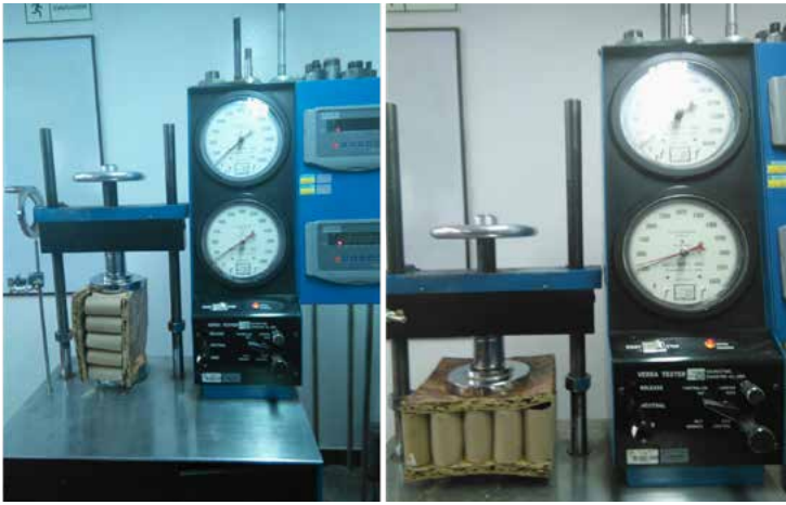
Figure 11. Equipment (hydraulic press) used to test horizontal and vertical load resistance
