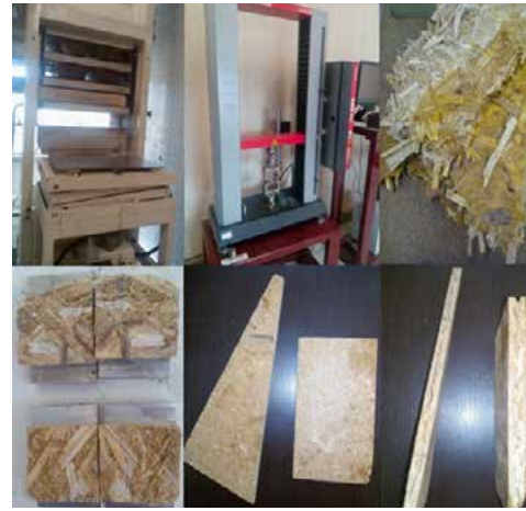
Figure 12. Manufacturing process of test samples and board
