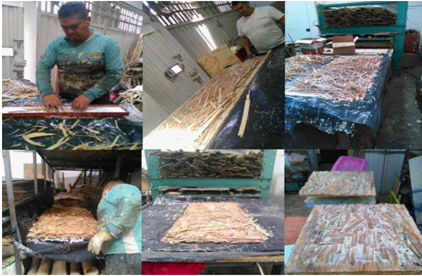
Figure 7. Manufacturing process of the OSB board, Muiskey company Source: Own elaboration, 2017, CC BY-ND.
