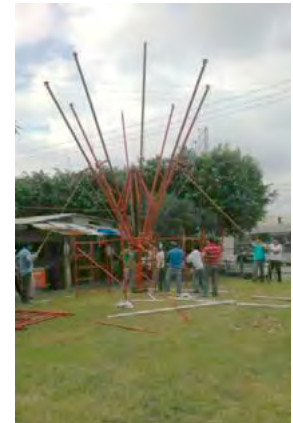
▶ Figures 64 to 66. A mobility test of the main arms without membrane was carried out to test the resistance of the winches and to identify the speed to achieve adequate resistance when deploying the transformable system.
