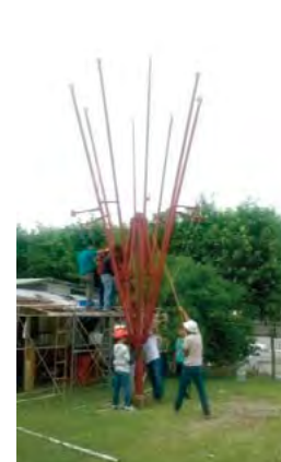
▶ Figures 64 to 66. A mobility test of the main arms without membrane was carried out to test the resistance of the winches and to identify the speed to achieve adequate resistance when deploying the transformable system.
